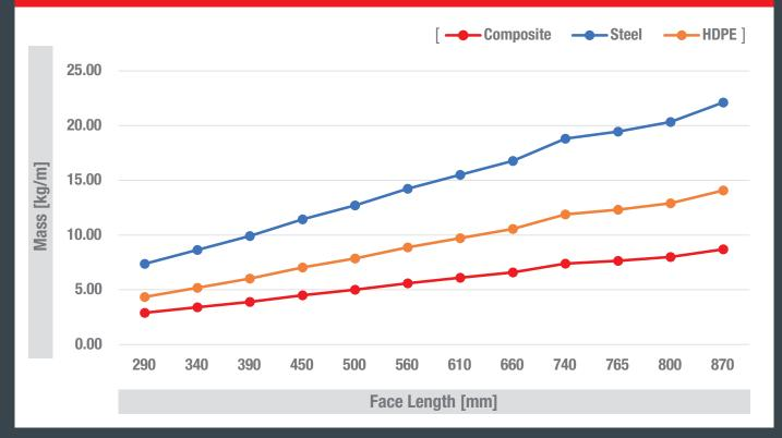
The Rulmeca Composite Roller offers a distinct mass advantage when compared to steel and HDPE rollers of equivalent length and diameter. Comparison based on solid shafting.
